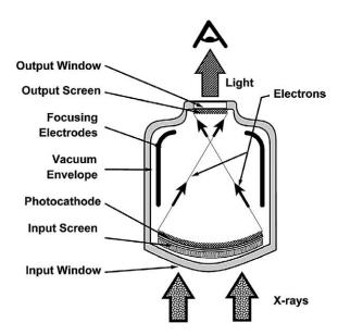
**Figure 8.** Diagram of an X-ray intensifier. The X-ray image passes through the input window and interacts in the input screen, converting the X-rays to a visible light image. The photocathode converts this light image to an electron beam image. The electrodes focus and accelerate the electrons that strike the output screen, producing the amplified light image of a much reduced size.
